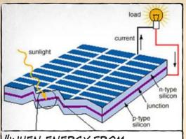
"WHEN ENERGY FROM SUNLIGHT REACHES THESE SEMICONDUCTORS, IT EXCITES THE ELECTRONS, CAUSING THEM TO FLOW. THIS FLOW IS ELECTRICAL CURRENT."
